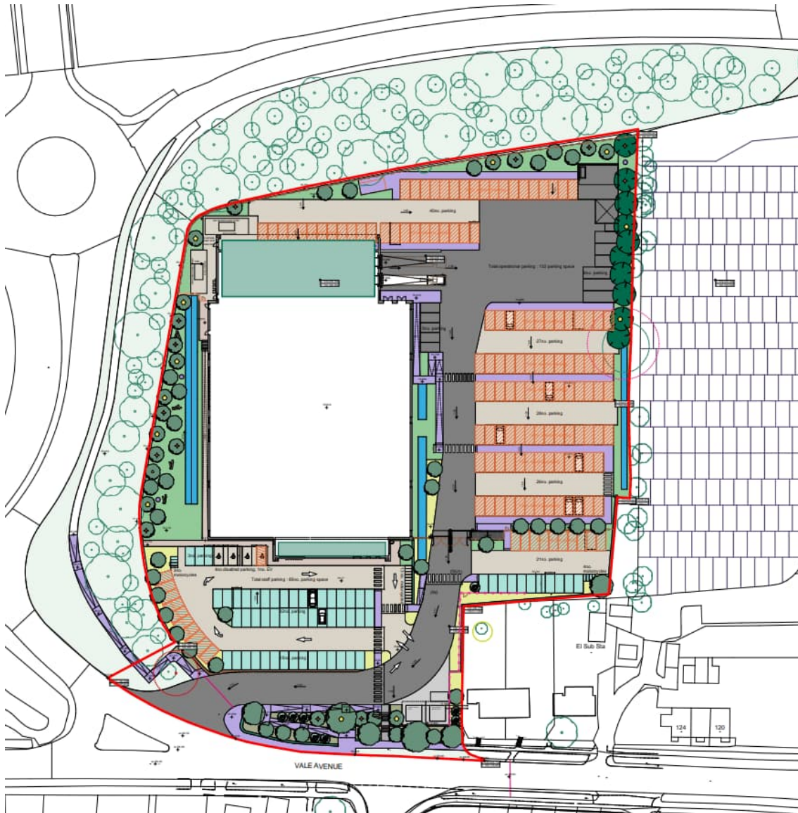
Figure 2.2: Site general arrangement plan
